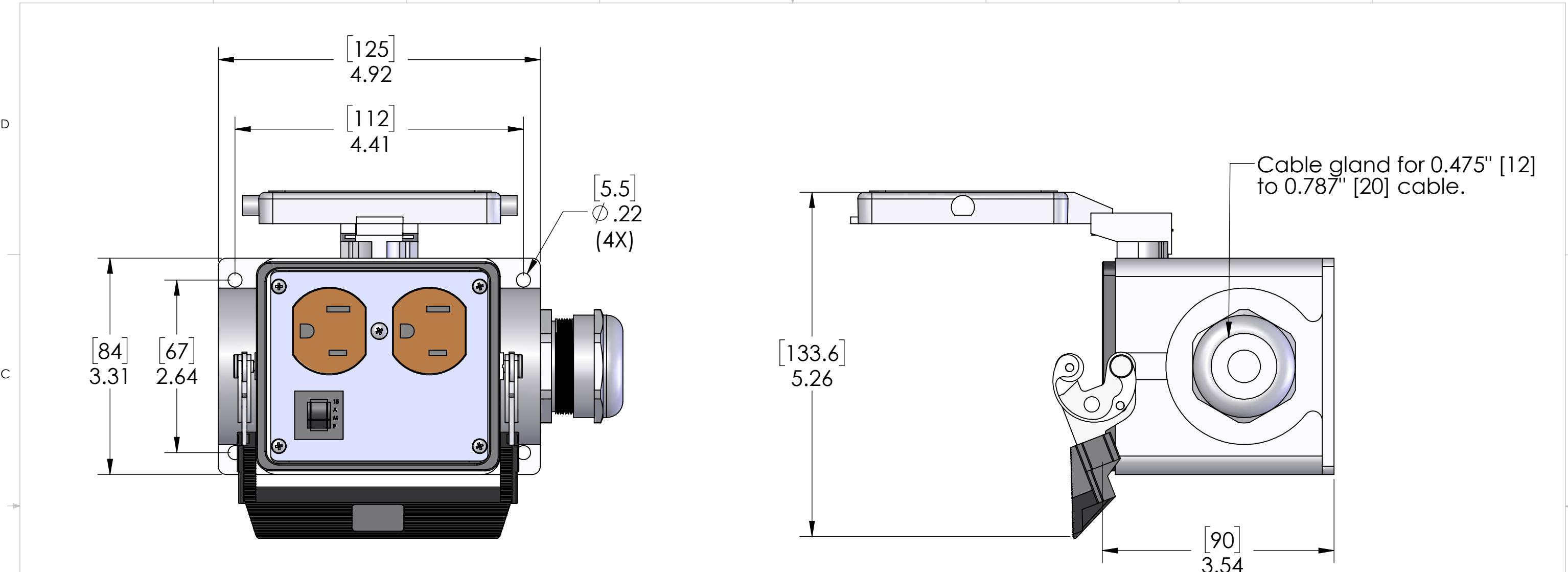
These devices shall be mounted on enclosures having adequate strength and thickness and with adequate spacing provided. Seal rating is based on mounting to a surface that is clean, flat and smooth.
