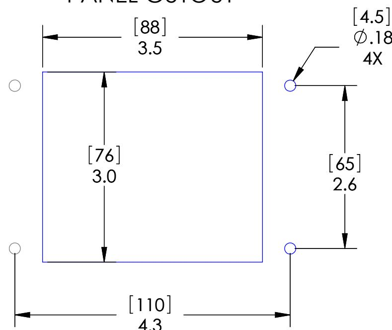
These devices shall be mounted on enclosures having adequate strength and thickness and with adequate spacing provided. Seal rating is based on mounting to a surface that is clean, flat and smooth.
