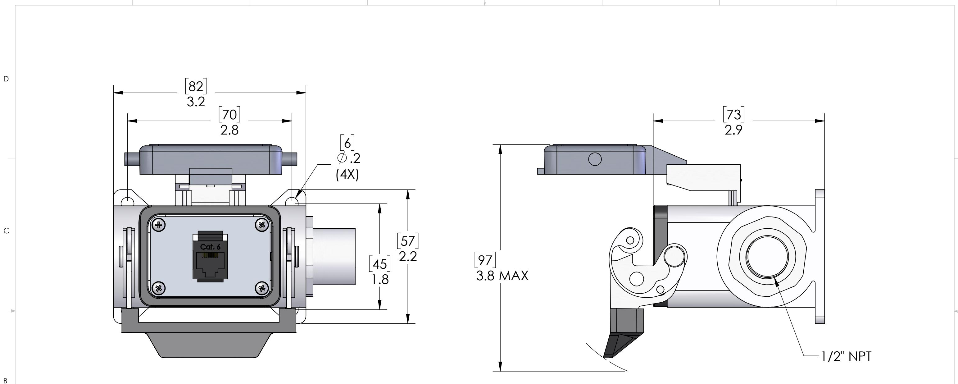
These devices shall be mounted on enclosures having adequate strength and thickness and with adequate spacing provided. Seal rating is based on mounting to a surface that is clean, flat and smooth.
